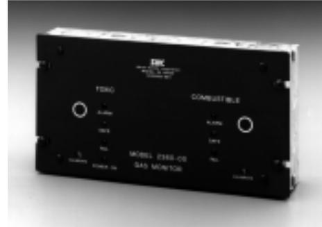
The monitor is mounted on a plate designed for installation into a customer supplied 3-gang switch box. A terminal strip on the component side of the electronic assembly board provides for easy connection of power input and relay output.
