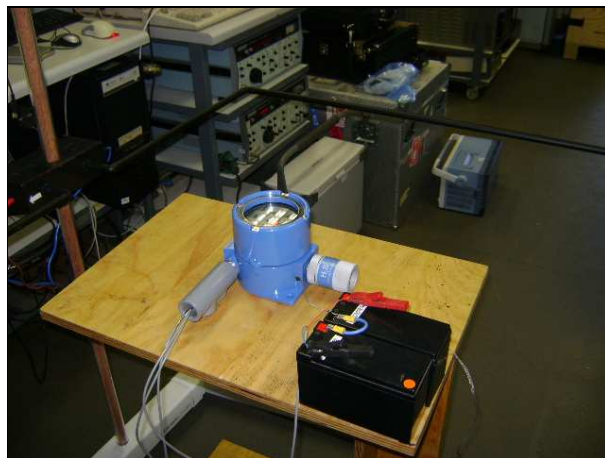
SANS / IEC 61000-4-8: Power frequency magnetic immunity test set-up
