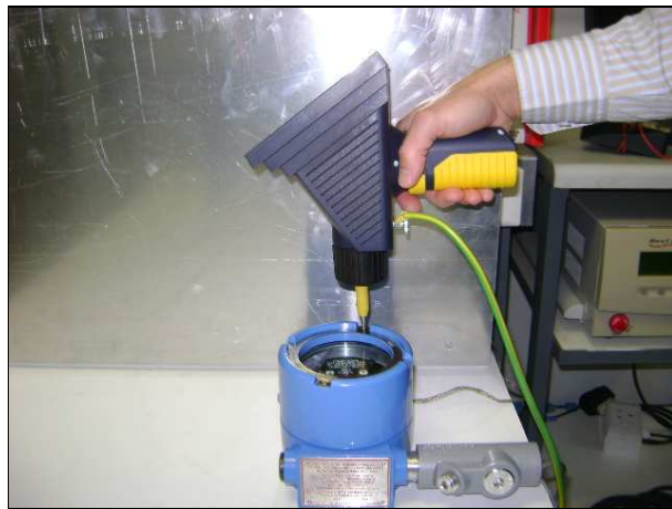
SANS / IEC 61000-4-2: Electro Static Discharge test set-up
