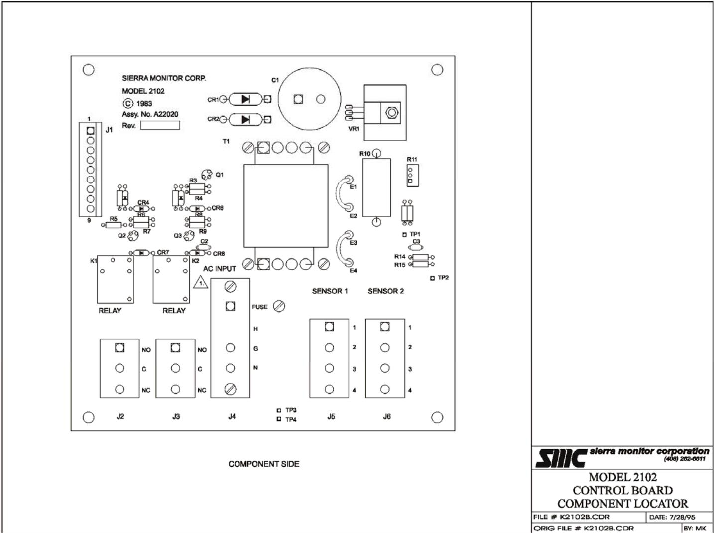
Figure 2 Component Locator
