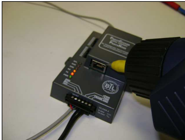
SANS / IEC 61000-4-2: ESD immunity test set-up
