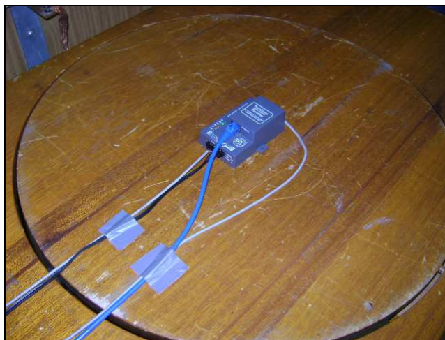
SANS 222 / CISPR 22: Conducted emissions test set-up
