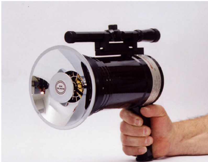
Figure 15: UV/IR Long Range Fire Simulator 20/20-311
